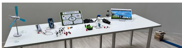
Figure 1. Overview of the experimental setup used in the hydrogen workshop, including renewable energy sources (solar panel, wind turbine), a PEM electrolyzer, a hydrogen fuel cell, and molecular models for conceptual visualization.
